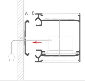
**9.** Secure the extrusion (B) against falling off by inserting the 4 mm plastic rods (F) into the guides and tightening them with M5 pressure screws (J) using the Allen wrench. Sink the pressure screws deep enough so there is room for end caps.
